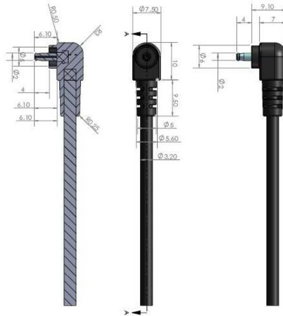
Electrical Connector Details
